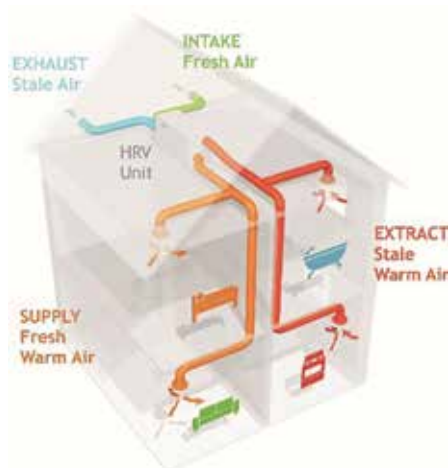
How a HRV/MVHR system works
